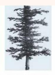
matrix acidizing of calcium carbonate shows an intricate network of wormholes created as the acid dissolved the rock. This network greatly enhances permeability around the welbore. providing necessary stimulation in many carbonate reservoirs.
